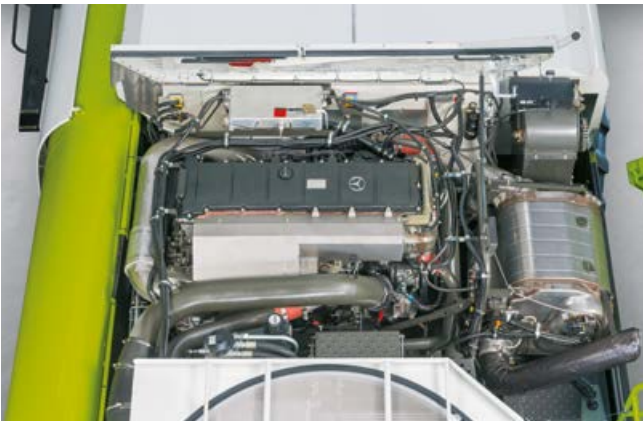
Mercedes-Benz OM 473 with 460 kW / 626 hp for LEXION 8700
