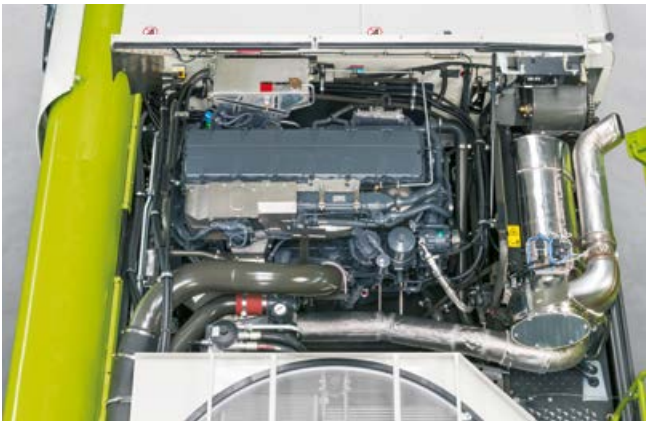
MAN D42 with 581 kW / 790 hp for LEXION 8900
