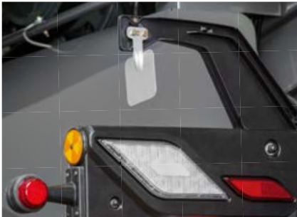
Sensor for automatic discharge direction adjustment
