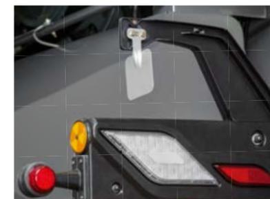
Sensor for automatic discharge direction adjustment
