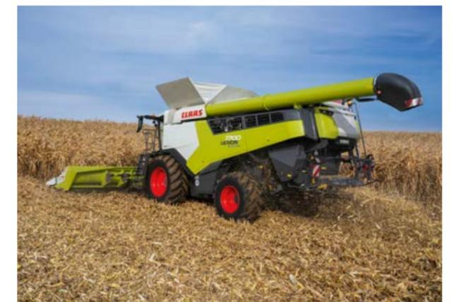
**Hydrostatic ground drive up to 40 km/h.**
