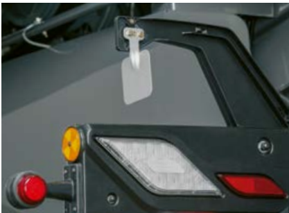
Sensor for automatic discharge direction adjustment
