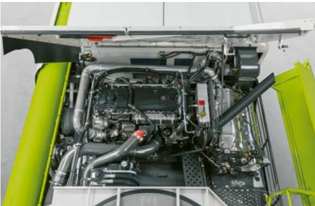
Mercedes-Benz OM 470 with 300 kW / 408 hp for LEXION 6700
