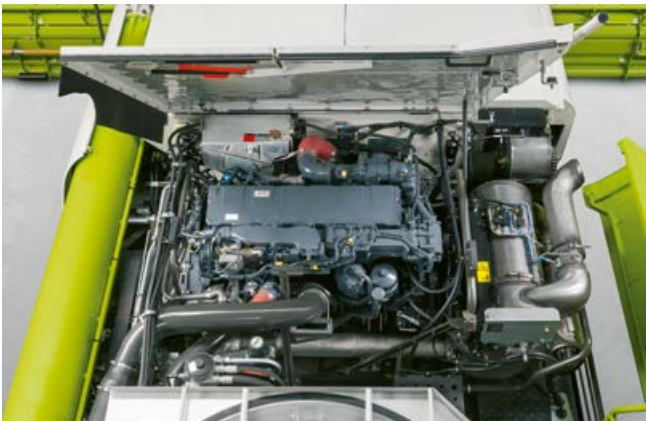
MAN D 26 with 373 kW / 507 hp for LEXION 6900
