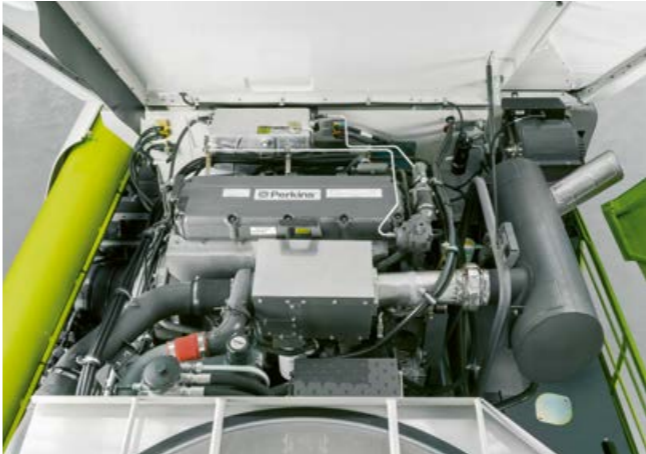
Perkins 2206D with up to 420 kW / 571 hp
