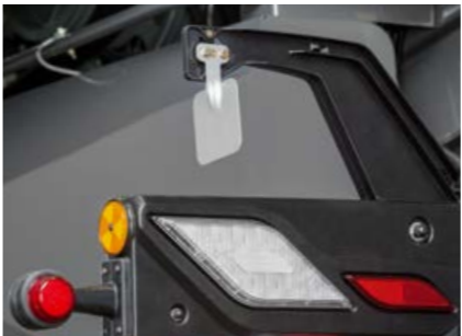
Sensor for automatic discharge direction adjustment
