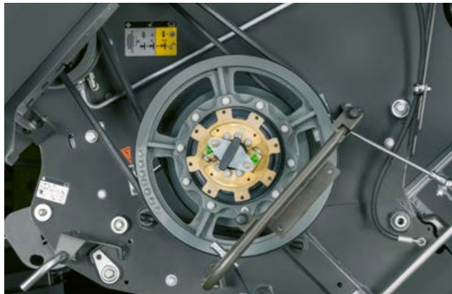
The speed of the straw chopper can be adjusted in line with your current task easily, quickly and without the need for tools.
