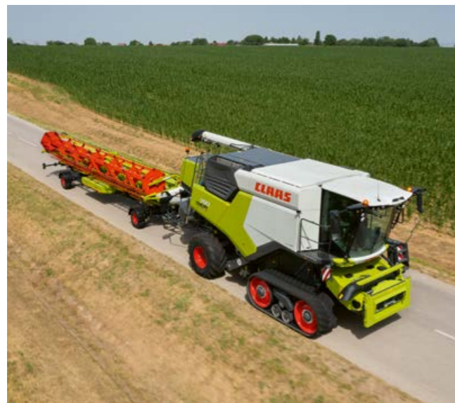
All TERRA TRAC crawler tracks are fully suited to road travel up to 30 km/h and provide a more comfortable driving experience than the wheeled machines.
