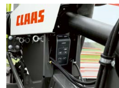
CEMIS 10 parking bracket for PLUS operation
