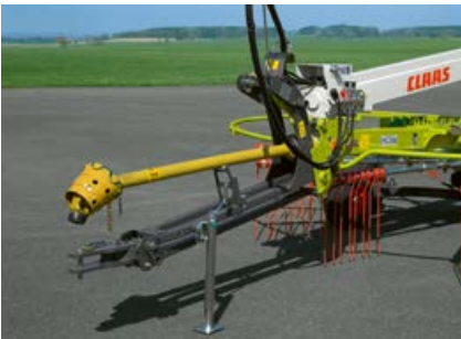
Parallelogram drawbar is optional on the LINER 700 TWIN and standard on the LINER 800 TWIN.
