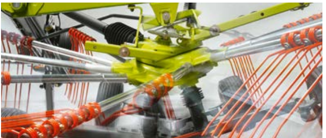
Fully floating cardan rotor suspension ensures that the rotors follow the ground contours independently of the tractor.
