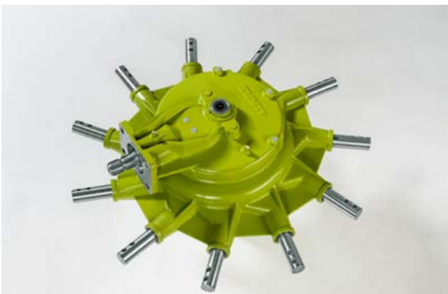
Eleven-arm rotor drive assembly in the LINER 320.
