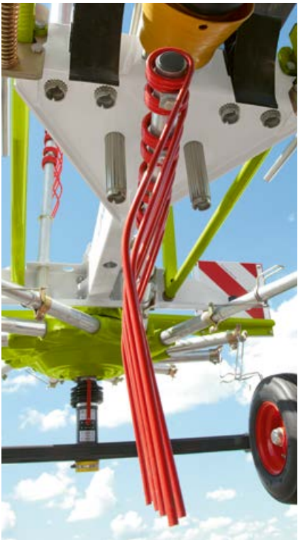
The 9 mm thick standard tines on the 450, 420 and 370 models are extremely robust, making them ideal for both hay and silage.
