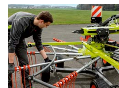
PROFIX tine arm attachment system
