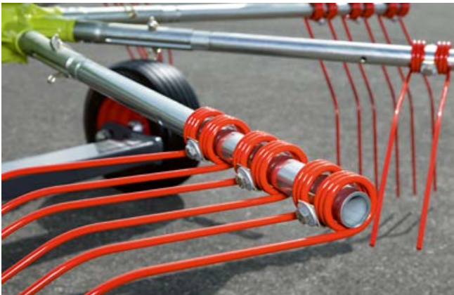
Tool-free tine arm removal.
